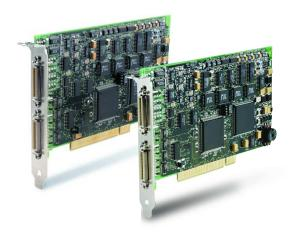
Our popular line of **KPCI data acquisition boards** allow fast, easy setup for a broad range of student lab applications. The DriverLINX<sup>TM</sup> software included provides a simple acquisition control interface.
